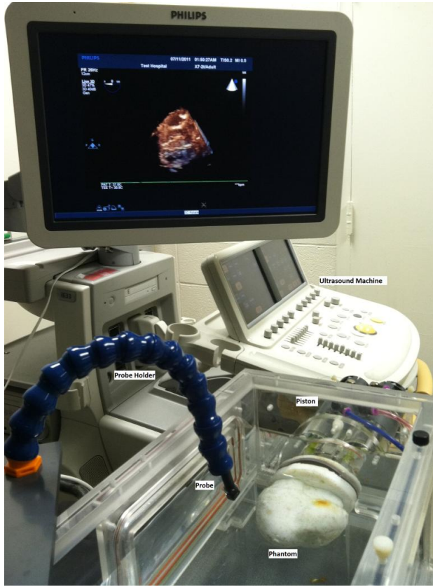
Fig. 1. Experimental setup showing the dynamic heart phantom in a water tank, a TEE probe secured within a probe holder and an ultrasound machine showing the phantom volume using a live 3D visualization scheme.
