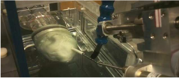
Fig. 3 Detailed view of the experimental setup showing the position of the TEE probe, beating heart phantom, and snake robot inserted into the heart at a point near the apex.
