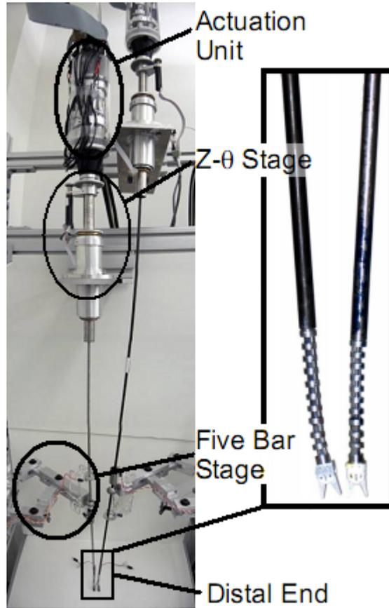
Figure 2: Snake Robot prototype
