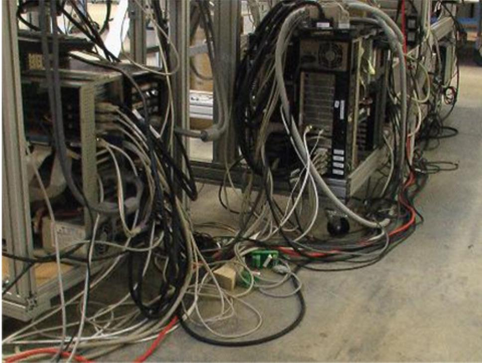
Figure 6: Original Snake Robot cabling with centralized I/O
