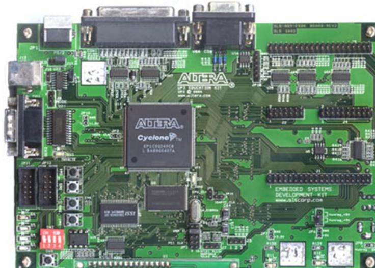
Figure 14: Altera UP3 FPGA development board
