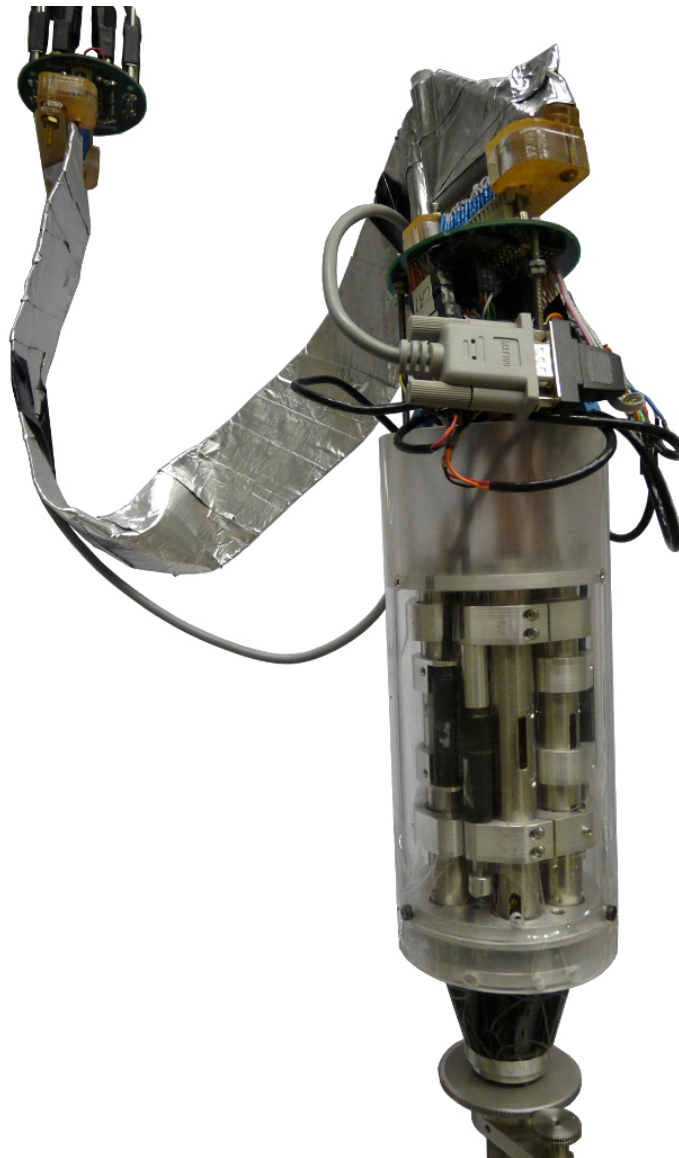
Figure A.4: Snake Robot actuation unit.
